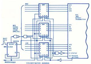
The figure shows a FIFO memory -- which can accept three BCD data bits and store 64 words -- used with the SER-DEX transmitter. Of course, a FIFO can be added for each additional BCD character that is desired. The system works in the following manner (a more-concrete functional description appears in the Appendix):
